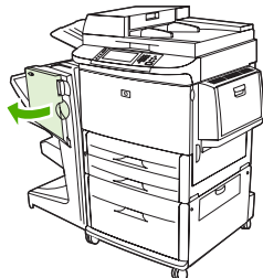
Figure 7-6 Load staples in the multifunction finisher (1 of 8)
